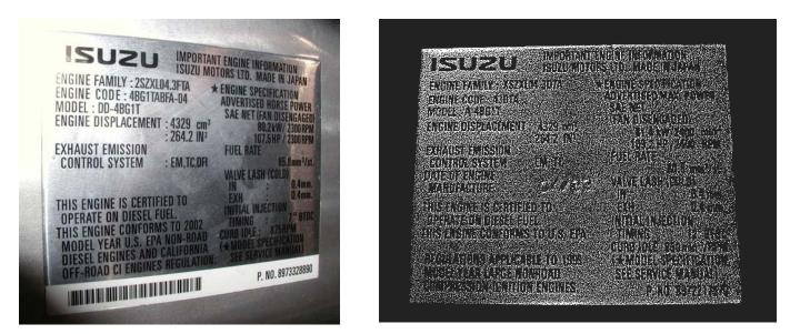
The EPA emission control label is affixed to the center of the injection pump cover, or on the upper side or top of the cylinder head cover. The label is often attached at a visible point on the equipment when the label attached to the engine is not visible due to the structure of the equipment.
